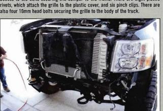
The stock bumper is held in place by six bolts that secure it to the frame. Retain the two dual bolts for use with the new bumper. I disconnected the electrical connector for the foglights and removed the bumper from the truck.
