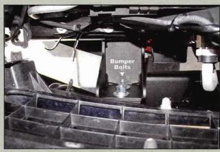
The grille must be in place before the bumper is installed on the truck.
