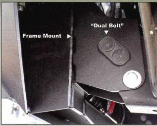
Before the bumper can be installed on the truck, the frame mount is attached to the frame using the OEM dual bolts and hardware provided by TrailReady.
