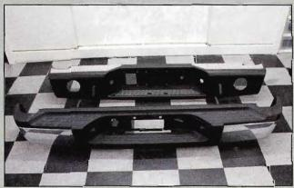
When placed side by side, TrailReady's rear bumper-with its all-steel construction, aluminum diamond-extruded top plate, D-ring, and light ports-makes the OEM look like it should be on a child's toy, not on a heavy-duty truck.
