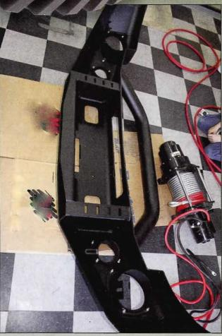
Even though the bumper is coated with Mini-Tex powdercoating, you still want to protect its finish by placing it on cardboard or other material while installing the accessories. The bumpers come with light buckets, mounting tabs, and ¼-inch Nylok nuts to secure the PIAA lights to the bumper.
