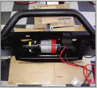
After installing the lights, it was time for the EP 16.5 winch. The bumper is predrilled to accept the 10x4-inch pattern for the roller fairlead. TrailReady's design allows for winches to be mounted foot forward or foot down. This is a feature not tound in many bumper designs.
