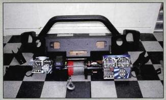
For the front of the truck, we will install TrailReady's extreme-duty front winch bumper made from ¼-inch and ¾s-inch steel with quad light ports for 4-, 5-, and 6-inch round lights, and D-ring mounts for 1-inch shackles. A Superwinch EP 16.5 winch, a pair of PIAA 520 ATP Xtreme White lights, and a pair of PIAA 510 Super White driving lights will be installed on the bumper.
